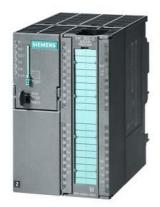
SIMATIC S7-300, FM352-5 with PNP output, High Speed Boolean Processor, for high-speed linking, 12 DI, 8 DO, 1 encoder interface for RS422 incr./SSI encoder
